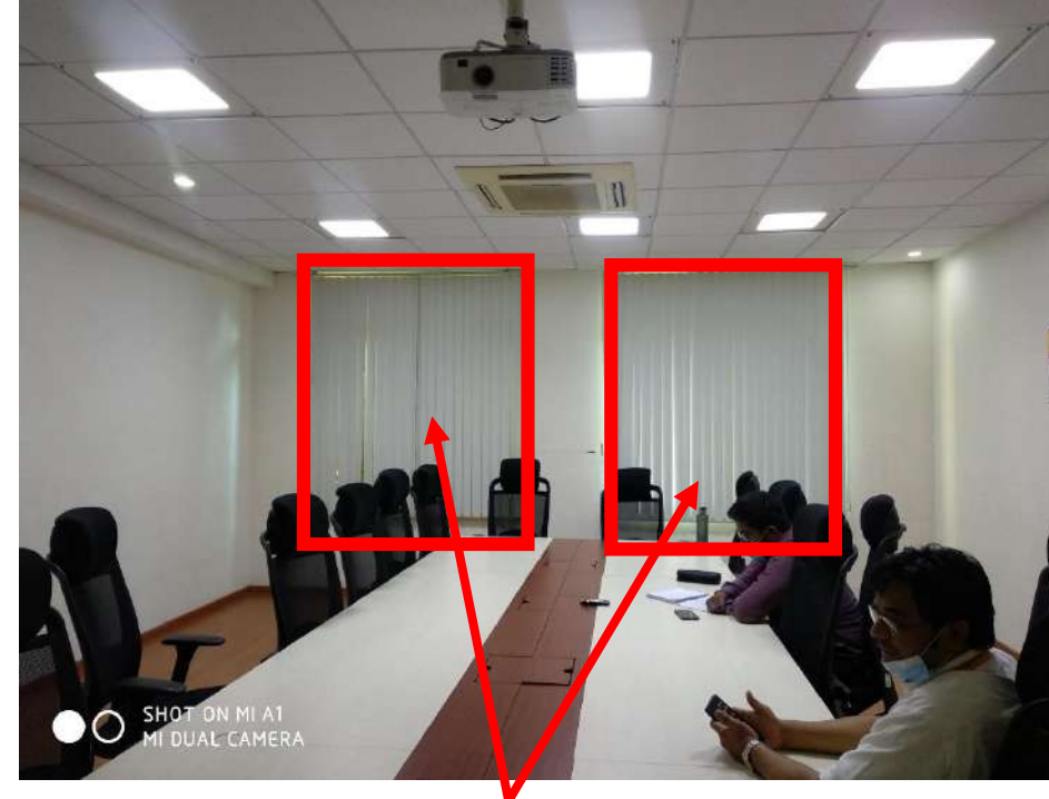
Image 5: No use of day lighting as drapes are shut during the daytime.
